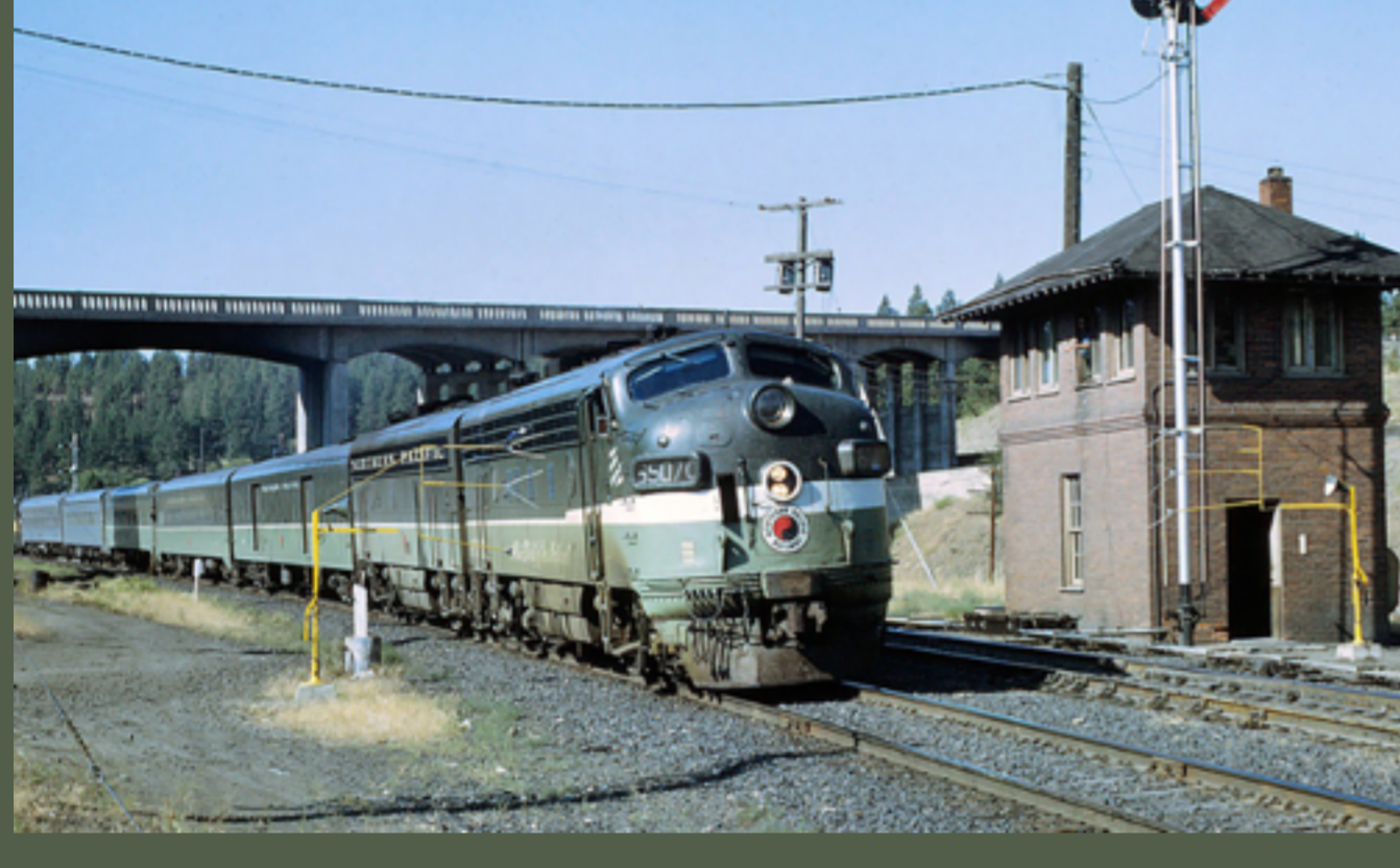
The tower operator gives a wave to the crew of EMD-built FP7 #6507, as Northern Pacific's eastbound Mainstreeter glides through Marshall on 27 July 1968. Check-out the train order hoops and the train order signal a clear indication that railroad's of the period were sometimes slow to adopt new technologies. (Doug Wingfield photo)
